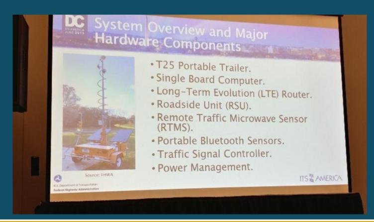
This portable trailer has multiple communication network interfaces:
