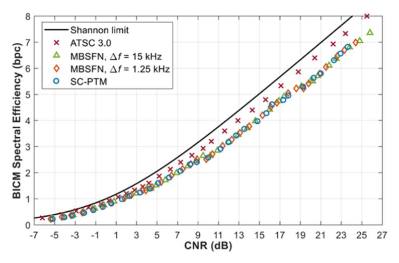
BICM Spectral Efficiency as a function of CNR for BLER=0.1% (SISO AWGN Channel)
